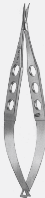
SS-689-11 Iris Micro Scissor Curved, Sharp Tips 10 mm Long Blades With Max. 5 mm Cutting Edge Overall Length 11 cm (4 ½")
