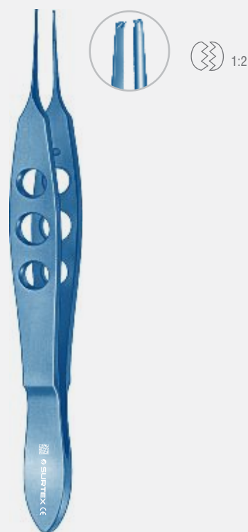
FR-732-10 T Bonn Corneal Forcep Very Delicate 1 x 2 Teeth With Tying Platform, 0.12 mm, Titanium Overall Length 10 cm (4")
