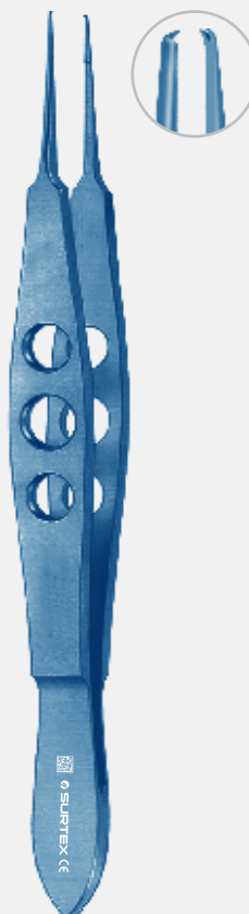
FR-750-01 T Castroviejo Suture Tying Forcep 1 x 2 Oblique Teeth, With Tying Platform 0.12 mm, Titanium Overall Length 11 cm (4 1/4")
