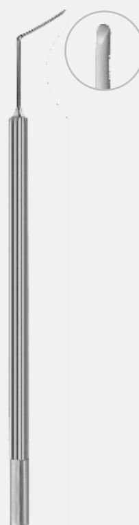
OP-717-12 Fukasaku LASIK Spatula 1.2 mm Wide Gently Curved Spatula With Round Anterior Edge and Flat Posterior Edge, Angled to Tip Length of 12 mm Overall Length 12 cm (4 3/4")
